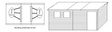
Lay each section of the roof on top of the shed, the shorter batons should be on the inside. Fix together the three sections using the 40mm screws as shown above.
