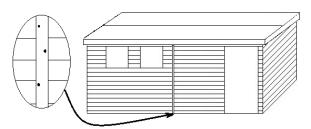
Place the joining strips over the front and rear joins in the shed panelsas shown and fix into place with the 30mm nails.
