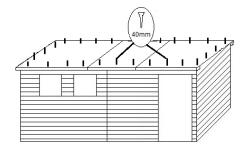
Align the roof so that it overhang s on all sides. Using the 40mm screws, fix the roof panel by screwing through it and into the framwork of the shed.
