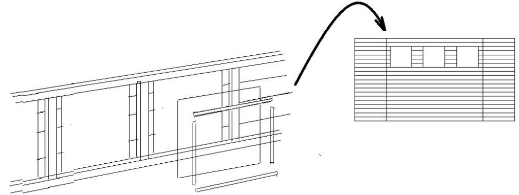
To fit the windows it is recommended that a waterproof sealant is applied around the edge of the glazing before fitting. From the inside of the building fit the styrene window into the frame and secure in place with the 4 strips of window bead. Fix the window bead to the window frame with 30mm panel pins .
