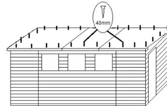
Align the roof so that it overhangs on all sides. Using the 40mm screws, fix the roof panel by screwing through it and into the framework of the shed.
