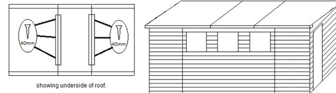
Lay each section of the roof on top of the shed, the shorter batons should be on the inside. Fix together the three sections using the 40mm screws as shown above.
