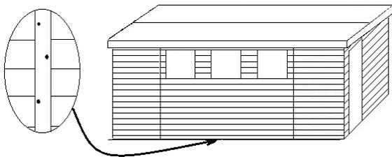
Place the joining strips over the front , rear and sides joins in the panels and fix into place with 30mm nails.
