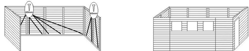
Once all of the side panels are in place, make sure that they are sitting squarely on the floor and fix each side panel to the floor as shown. Use 60mm screws and ensure that the screws go through the floor into the bearers.
