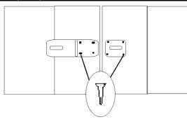
Position the two parts of the hasp & staple across the join in the doors. Make sure that that they are both level and will fit together when fixed into place.
