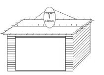
Lay the roof felt with an overhang all round. Fold down the felt at the front and secure using the 10mm clout nails. Tension the felt over the roof and secure to the rear of the roof. Space the clout nail approx. 15cm. Follow the above steps for the sides of the roof. Once the felt is secure trim off any excess.
