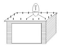
Lay the roof on the shed as shown. Using the 40mm screws, fix the roof into position by screwing through the roof panel into the internal framework of the shed.
