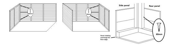
Secure the rear and side panels together as shown below, using 60mm screws. Note that the framework of the panels rests on the floor with the cladding over hanging. Continue until all sides including the front panel are in place and fixed together.
