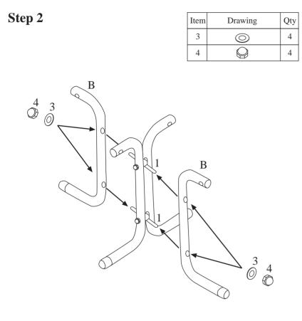
Attach each leg to cross shaped bolt (1) with washer (3) & round top nut (4). Assemble as shown.
