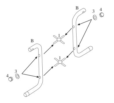
Attach each leg (B) to cross shaped bolt (1) with washer (3) & round top nut (4). Assemble as shown.
