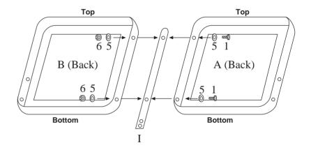
Place the flat metal bar (I) in one end and connect two back panels with bolt (1) and washer (5) and nut (6) on other side.
