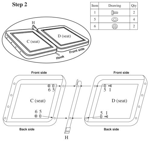
Place the flat metal bar (H) with hook in one end and connect two seat panels with bolt (1) and washer (5) and nut (6) on other side.
