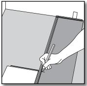
[3] To measure a shorter plank section for the end of the first row, place the final plank face down with the short tongue of the end seam toward the wall. Remember to allow for a minimum 1/4" expansion space. Draw a pencil line where this plank is to be cut.
