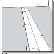
[8] After you have connected three or four planks of the second row in this manner, you can now go back and lock the side seams of the first planks into position.
