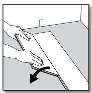
[6] Place the short start board for the second row firmly against the side seam of the start board in the first row, but do not fold it down to lock it into place yet.
