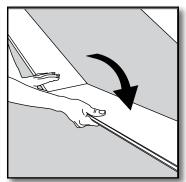
[2] To start the first row, press the end seam of the second plank at an angle to the end seam of the first plank, and then lock them together by laying the plank down. Complete the entire first row in this manner.
