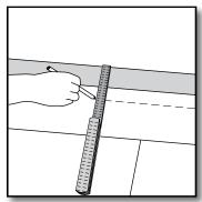
[11] If the starting wall is uneven, the planks must be adapted to its contours. You can scribe the contour of the wall onto the first row of planks by using a ruler and a pencil to follow along the contour of the wall. Do not forget to allow for the minimum 1/4" expansion space from the wall. Disassemble the first row, cut the planks along the line you have drawn, and then reassemble. You must still use the spacers to maintain the expansion space along this wall.
