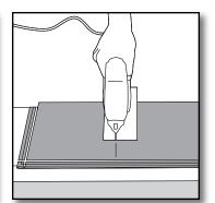
[4] Place the plank face down on the work surface and cut to size with a power saw. If you are using a hand saw, use a fine-toothed blade and cut the planks face up.
