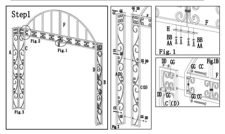
**Fig.1:** Unfold the Side Panel F and keep it flat by the Connecting Bar H, the Bolt AA and the Washer BB. See Fig.1A
