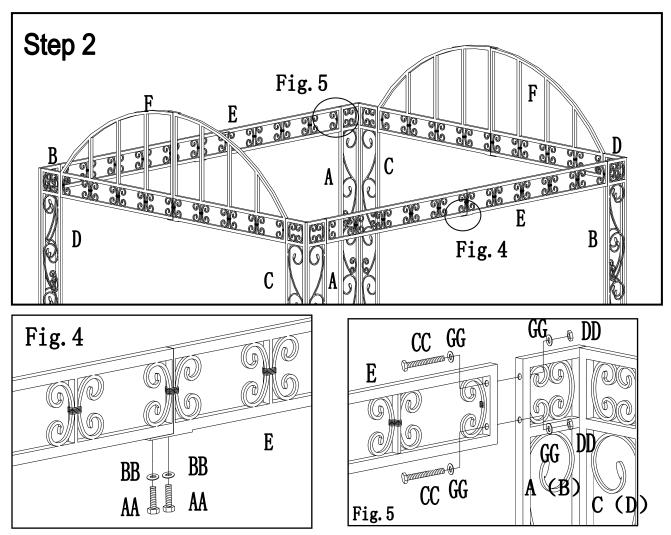
**Fig.4:** Unfold the Beam Screen E and keep it flat by the Bolt AA and Washer BB. See Fig.4 **Fig.5:** Attach the Beam Screen E to Post Screen A and Post Screen B with Bolt CC, the Nut DD and Washer GG. See Fig. 5.
