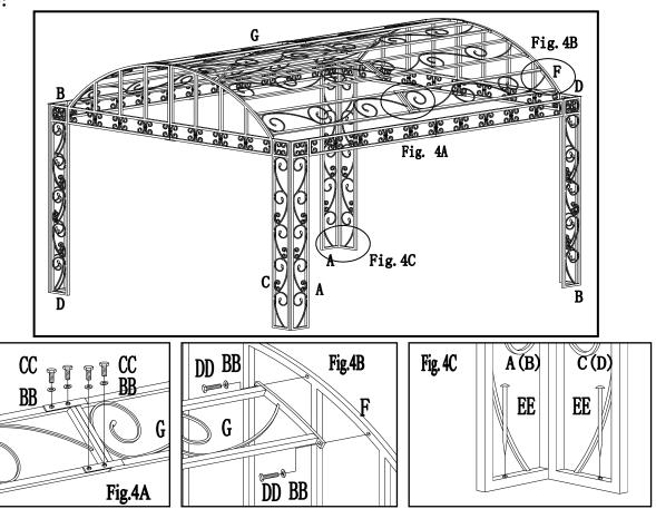
**Step 6:** Unfold Top Screen (G) and securely attach it with Bolt (CC) and Flat Washer (BB). See Fig.4A. Repeat until all 6pc of Top Screens (G) are assembled.
