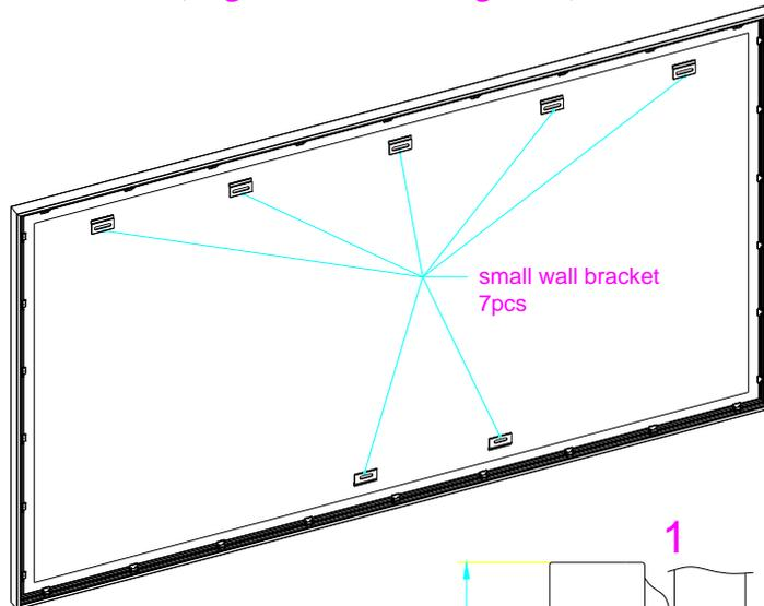
Position the screen with the attached surface onto the top wall bracket as shown in (fig.8). Push down at the center of the bottom frame rail to hook onto the lower wall bracket
