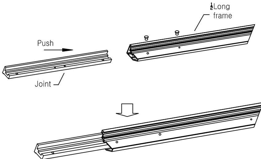
2. Insert the other horizontal frame piece to the joint connector and then fasten it with 2 screws.
