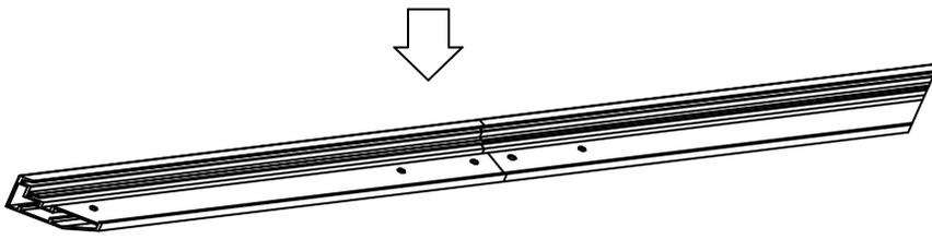
Please do not tighten the screws completely, to make sure the frame piece lines up correctly.
