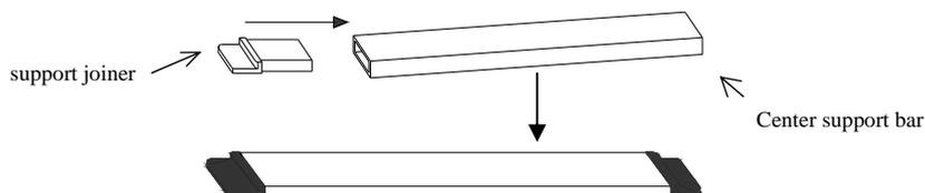
2. Insert the Center Support Bar into the groove on the back of the frame with the bottom end near the approximate center point of the frame and place it in at an angle so that both ends of the bar are in alignment with the groove. (see Fig. 8 below for details).
