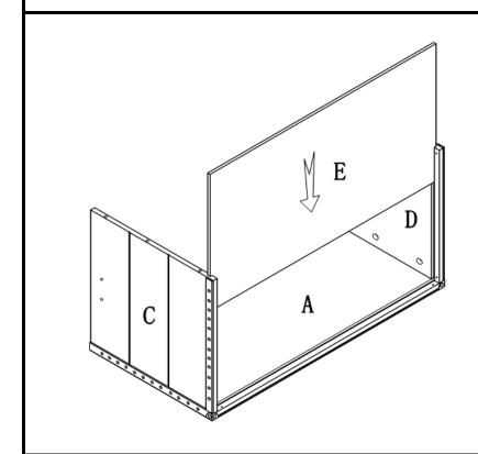
Step 2: Insert bottom panel (E) to the groove side panel as shown.
