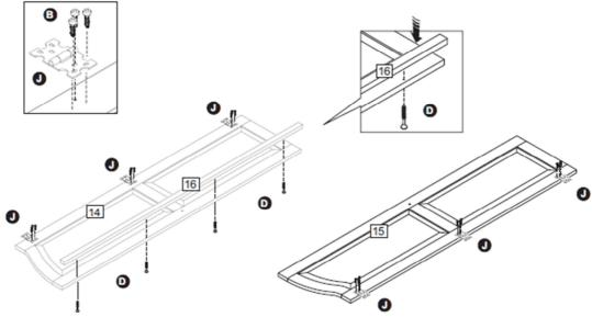
**Step 14:** Position the doors and secure using hardware part B and a screwdriver (not provided) **DO NOT use any power tools as this may damage the frame and will invalidate any claim**
