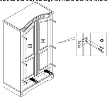
**Step 15:** Attach hardware part H using hardware part G and a screwdriver (not provided)
