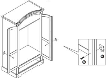
**Step 16:** Secure hardware part K using hardware part B. Insert hardware part L ensuring they are level then push the door against it to create 2 small marks. Secure hardware part L where the two marks are, using hardware part B. You will need to use a screwdriver (not provided)
