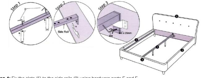
**Step 4:** Fix the slats (5) to the side rails (2) using hardware parts E and F **DO NOT use any power tools as this may damage the frame and will invalidate any claim**
