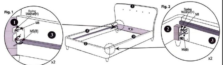
**Step 3:** Fix the centre legs (7) to the centre rail (4) using the M5 Allen key, then attach the rail to the headend (1) and footend (2) using hardware part A and the M4 Allen key
