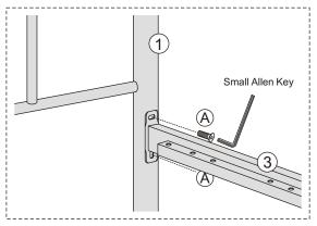
IMPORTANT Do not tightly secure the screw yet before assembling the Side Frame (Step 2)
