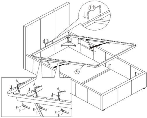
**Step 4**: To attach the pull strap (12) place it beneath the frame, then pull the strap on the inner side of the frame through the strap on the outer side to form a knot. Place hardware part K onto each slat (13) then push firmly into the metal frame (9).
