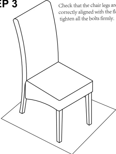
Check that the chair legs are level and correctly aligned with the floor then tighten all the bolts firmly.
