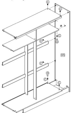
Step 8: Position the hanging rail (18) and attach the left panel (4) using hardware parts C and D with a screwdriver (not provided).
