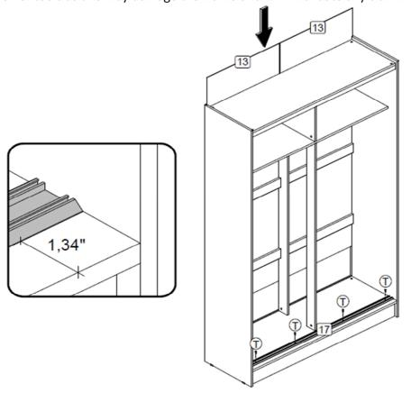
Step 10: Secure the back panels (13) using hardware parts I and L with a small mallet (not provided). Attach the top plinth (3) using hardware part P with a screwdriver (not provided).
