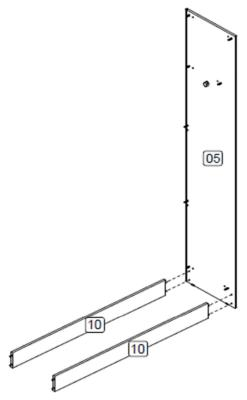
**Step 7**: Join the assembled inner frame section to the assembled side frame section using hardware parts C and D with a screwdriver (not provided).
