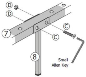
Step 6: Adjust both of the side supports (5) into inner direction until the screws reach the end of the hole as shown. Tighten the screws for the side supports and the mid support.
