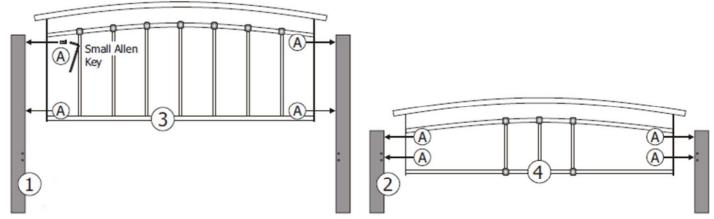
Step 2: Fix the side support (5) to the headposts (1) and footposts (2) using hardware part A. DO NOT use any power tools as this may damage the frame and will invalidate any claim.
