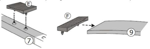
Step 8: Place the slats (9) into hardware part E then press hardware part F firmly into the side supports (5). DO NOT use any power tools as this may damage the frame and will invalidate any claim.
