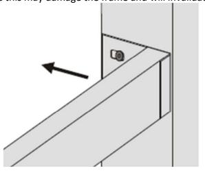
Step 7: Press hardware part E into the mid support (7) then place hardware part F onto an end of every slat (9).
