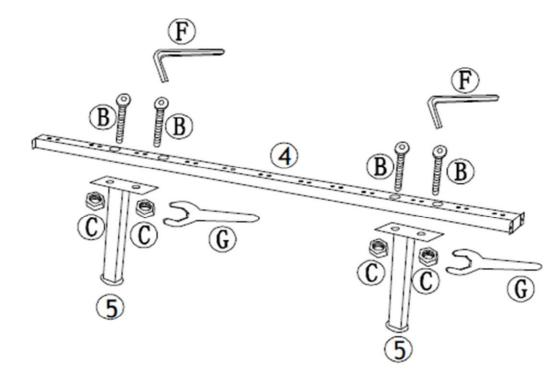
Step 3: Attach the side rails (3) to the headend (1) and footend (2) using hardware parts A, D, E and F. Then attach the centre rail (4) using hardware parts A and F.
