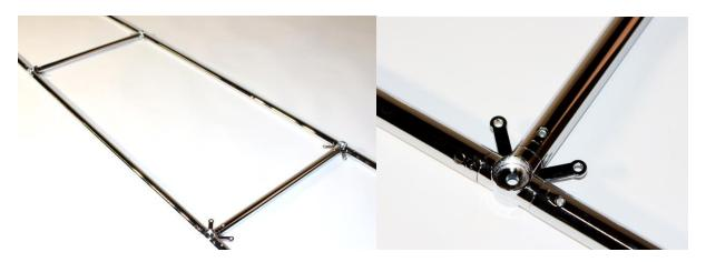
Adjust left side and right side, then place the tubes so you may lock in on both sides with one twist per tube. Make sure then the holes in the steel tubes are facing inside the framed box to place later on the screws.
