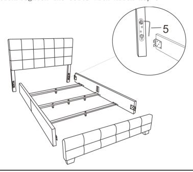
Step 4:Place the three support rail to the U shape, adjust the legs(k) into a same level.
