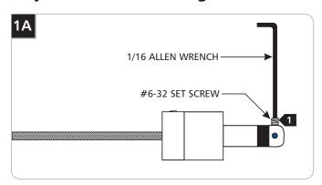
Back out (**DO NOT REMOVE**) the #6-32 set screw on tip of the connector with the provided 1/16 Allen wrench.
