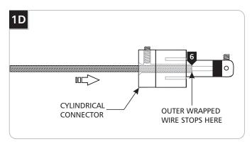
Feed and push the coaxial cable into the cylindrical connector. The coaxial cable will come to a stop point after being inserted 3/4" into the cylindrical connector.
