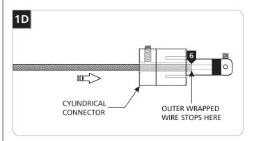
Feed and push the coaxial cable into the cylindrical connector. The coaxial cable will come to a stop point after being inserted 3/4" into the cylindrical connector.
