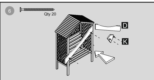
Place the barge boards to the roof so that the bottom of the curve is in line with the top of the roof and they meet at the apex. Fix each in place using 4x40mm screws,
