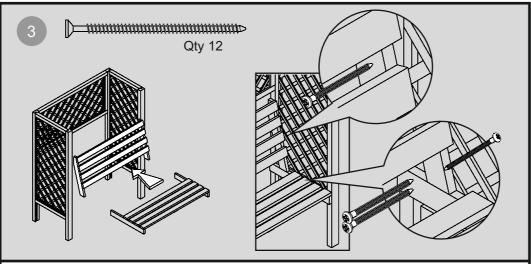
Place the bench seat between the two sides so that it is tight and the bottom of the bench is 378mm from the ground. Fix this in place using 2x60mm screws to fix each end to the posts of the
