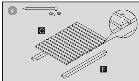
Place the roof slat section on to two of the shaped battens as shown. Make sure these are flush on both sides and in line with the un-notched end. Fix each slat in place using a 40mm nail on each
