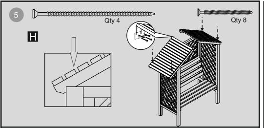
Fix the two roof sections together and secure using the metal plates and 8x40mm screws as shown.
