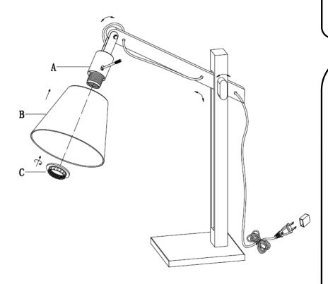
1.. Place the shade (B) onto socket holder (A) and screw it by socket ring (C).
