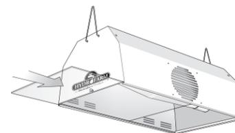
Rotate the tab upwards and carefully slide lens in from the end of the reflector. Rotate the tab down to retain the lens.
