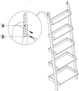
DO NOT FULLY TIGHTEN all screws and bolts until the product is leaning against the wall.
