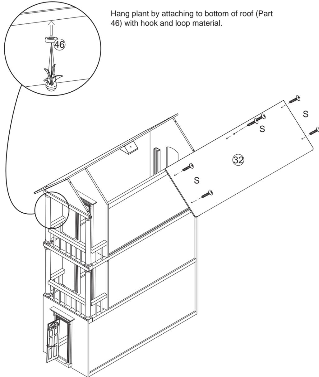
Hang plant by attaching to bottom of roof (Part 46) with hook and loop material.
