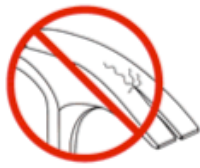
Crack in claw section
