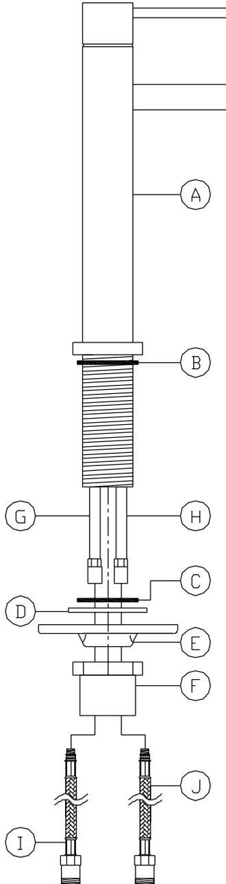
1. Place the upper seal (B) onto the base of the tap (A).
