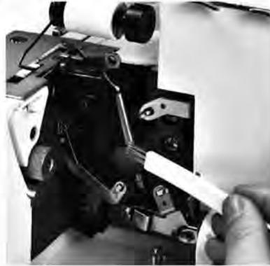
Use the lint brush from the accessories to remove lint from the needle plate, the upper and lower knives and looper area.
