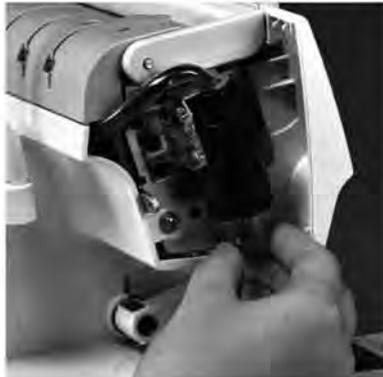
Push the bulb into the socket, give it a half-turn in a counter-clockwise direction and remove it .
