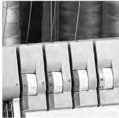
**Adjusting the thread tension**
