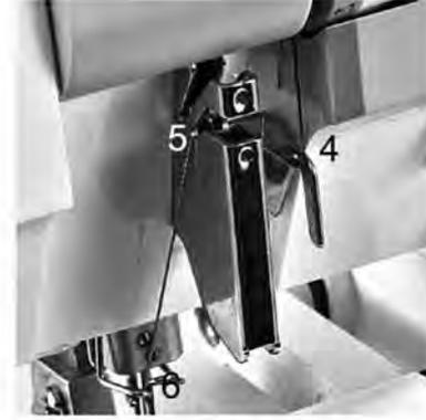
**Note:** The thread must run through the lower slot in guide 5.
