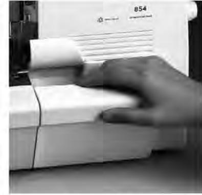
Press against the lower part of the container until the lower tabs snap into the lower slots of the looper cover.
