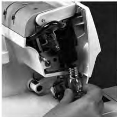
Insert a new bulb (max. 15 Watt) into the socket and rotate it until the two cams of the bulb lock in. Push the bulb into the socket, thereby rotating it in a clockwise direction until it is firmly in place. Replace the sewing lamp cover and tighten the retaining screw.
