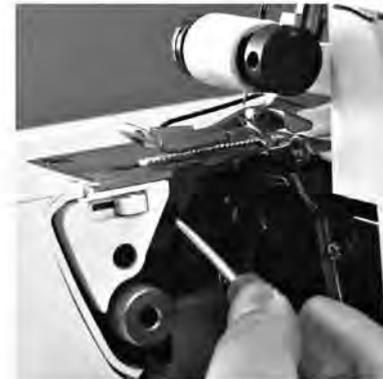
**Insertion:** Insert a new lower knife into the recess provided and tighten the retaining screw. Engage the upper knife and close the looper cover.
