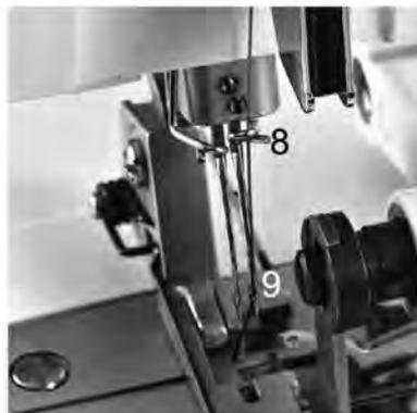
Pull about 10 cm of thread through the looper and lay it to the left underneath the sewing foot.
