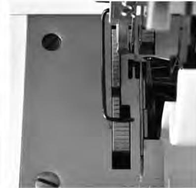
Stitch finger **A** will be pushed forward. All standard overlock seams can be sewn with this adjustment.
