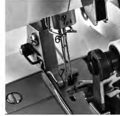
Pull about 10 cm of thread through the needle eye and lay it to the left underneath the sewing foot.
