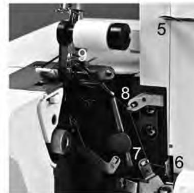
Insert the thread along the path marked in pink through guides 5 to 8.
