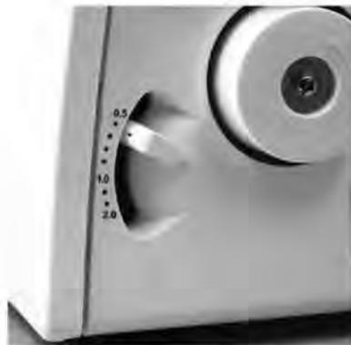
If differential feed adjustment lever 30 is set to 0.5, the front feed dog moves half as fast as the rear feed dog, i.e. the front feed dog feeds through only half as much fabric as the rear feed dog.
