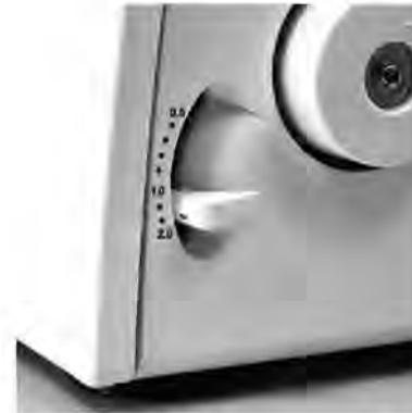
Set differential feed adjustment lever 30 to 2.0 so that the front feed dog moves twice as fast as the rear feed dog, i.e. the front feed dog feeds through twice as much fabric as the rear feed dog.
