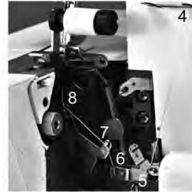
Insert the thread along the path marked in yellow through guides 4 to 8.
