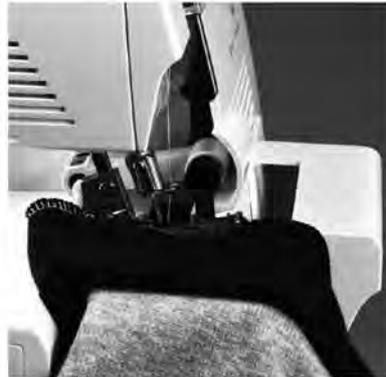
The free arm is particularly useful for sewing tubular items such as trouser legs and sleeves. Insert the article over the free arm.
