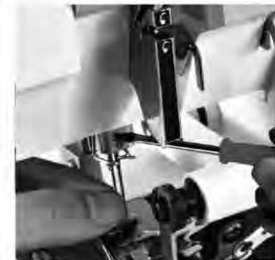
Loosen the needle fastening screw (without removing it completely) with the small screwdriver included in the accessories and remove the needle in a downward motion. Insert a new needle into the needle holder **with the flat side to the rear** and retighten the respective fastening screw.
