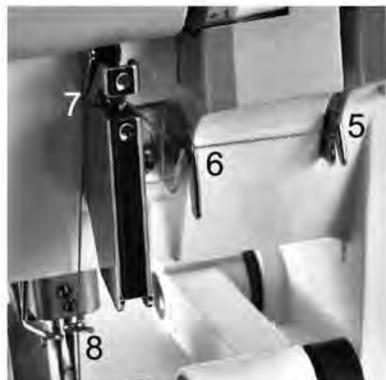
**Note:** The thread must run through the upper slot in guide 7.
