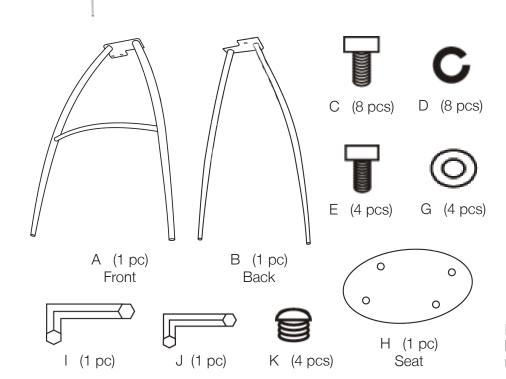
During assembly, hand tighten screws only. When all screws are in place, then tighten completely. 2 С C D D C. 8 3000
