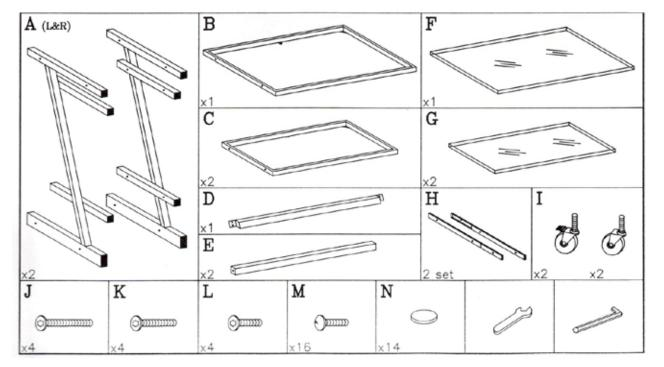
During assembly, hand tighten screws only. When all screws are in place, then tighten completely.
