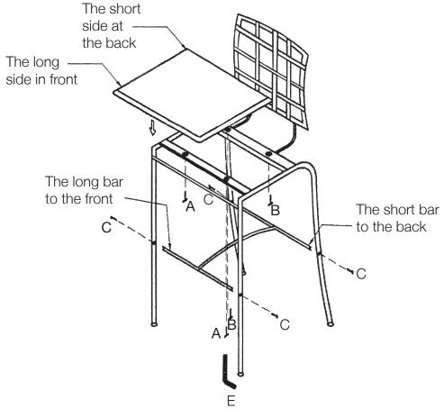
During assembly, hand tighten screws only. When all screws are in place, then tighten completely.
