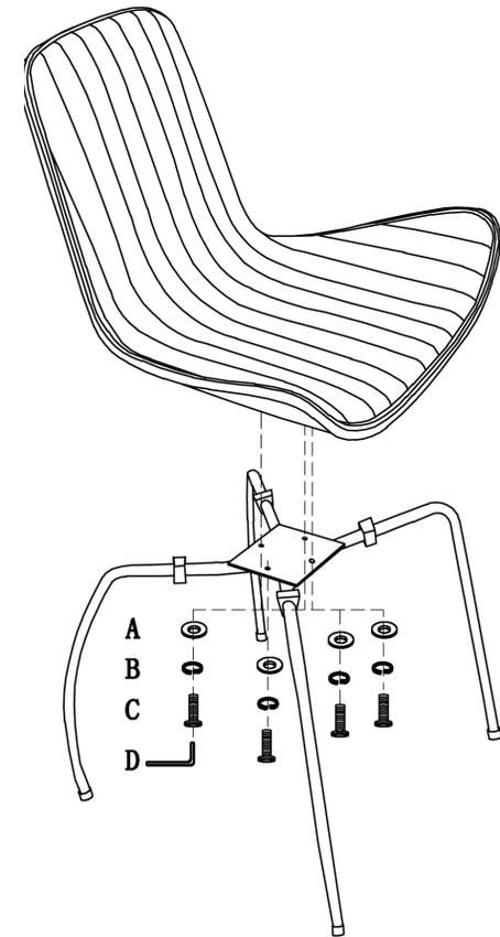
During assembly, hand tighten screws only. When all screws are in place, then tighten completely.
