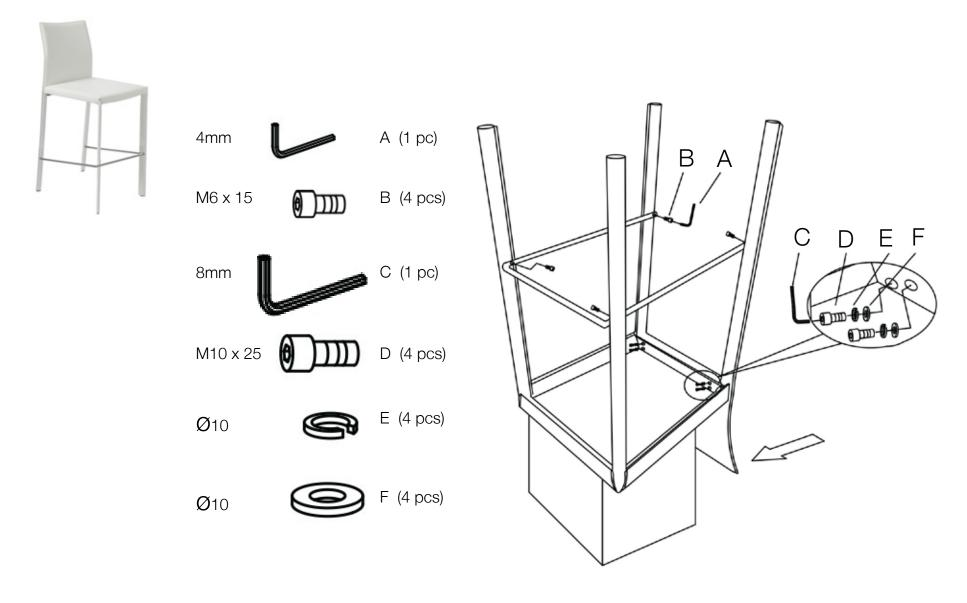
During assembly, hand tighten screws only. When all screws are in place, then tighten completely.
