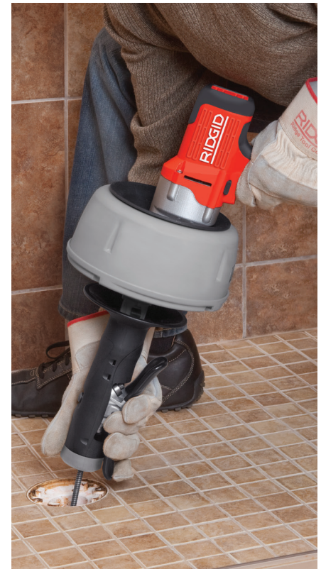
The 3/8" cable in Model K-45AF-5 and K-45AF-7 extends machine's capacity to 2 1/2" drain lines.
