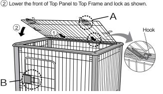
1) Place the rear hooks of Top Panel on Top Frame as shown.
