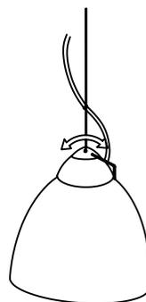
Loosen the allen screw, then rotate assembly into a new position that will level the glass shade.
