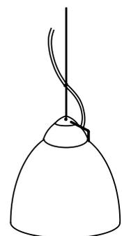
Hold the shade in it's new position, then tighten the allen screw firmly. Release the glass shade and visually confirm that it is now level.
