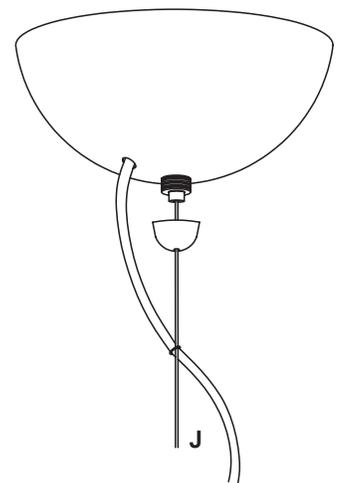
**Overtightening can cause the Retainer to be difficult to unscrew. If this occurs, usually rotating the canopy counter-clockwise will help to unlock the Retainer.**
