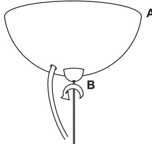
2. Prior to mounting fixture to ceiling, cord must be cut to length. Measure the overall length of pendant drop, then add 25% to allow for shaping of the cord. Cut off excess cord then strip back outer jacket about 4" in length. To move the Strain Relief (I), simply pinch together and slide down the cord.
