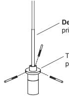
**Decorative Sleeve**, must be installed prior to installing cord into the ceiling canopy.
