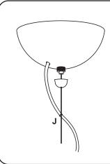
6. Replace the Canopy as shown and secure with the Retainer. Tighten the Retainer enough to hold the Canopy to the ceiling but do not overtighten. The cord can now be shaped by positioning the Cord Rings (J) along the cable as desired.
