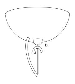
1. Carefully unpack parts. Remove the Canopy (A) from the Mounting Plate by unscrewing the Retainer (B). Fully remove the Retainer from the threaded nipple, then pull the canopy from the Mounting Plate.
