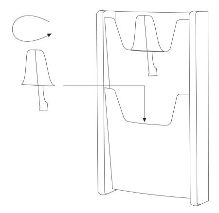
Twist Divider 1/8 turn to fit between pockets. Then twist straight and snap divider down into top of the pocket.
