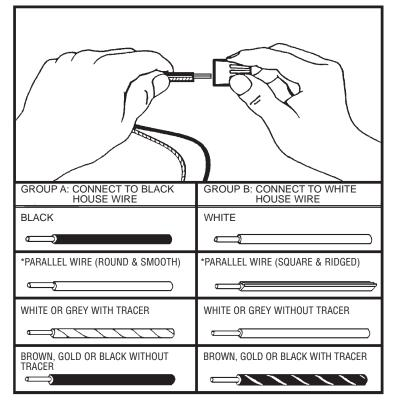
\*NOTE: When parallel wire is used, the tracer wire is square shaped or ridged, and the less tracer wire is round in shape or smooth. (Seen best when viewed from wire end.) To separate wires, grasp the ends of each wire and pull apart.
