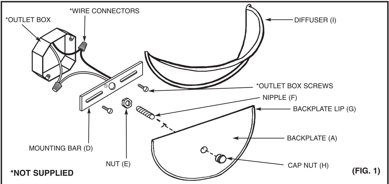
IF SUPPLY WIRES ARE LOCATED WITHIN 3" OF BALLAST, USE WIRE RATED FOR AT LEAST 90°C.
