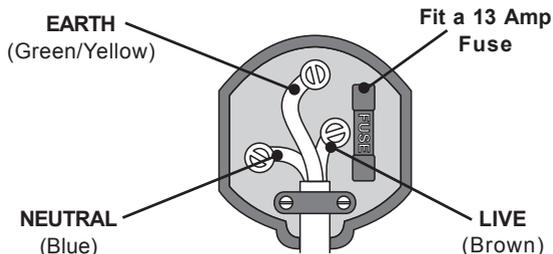
**Ensure that the outer sheath of the cable is firmly held by the clamp.**
