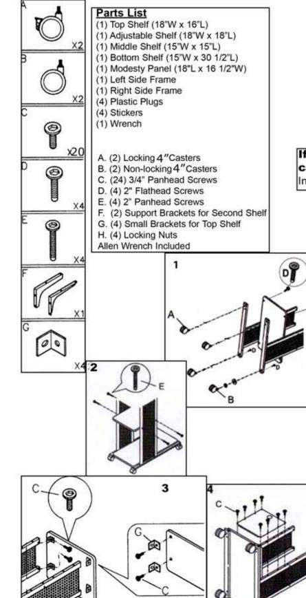
6. Take adjustable shelf (18" x 18") and attach the (2) large "L" support brackets (F) making sure that the smooth side of
