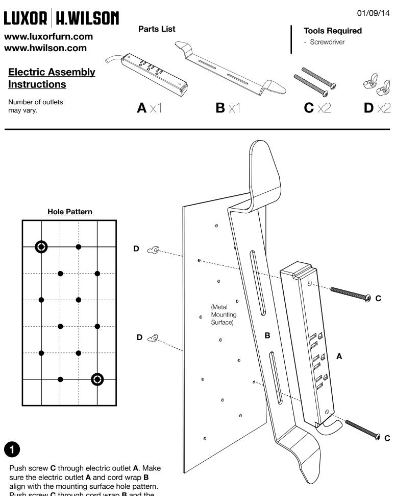
Push screw **C** through cord wrap **B** and the mounting surface screw holes. Use wing nut **D** and screwdriver to fasten.
