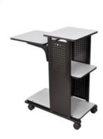
Important Assembly Tip: When assembling a WPS4E OR a WPS4CE, do not tighten the screws all the way down. Leave them approximately 1/2 turn out. When unit is fully assembled, tighten screws all the way. This will allow the unit to line up correctly.
