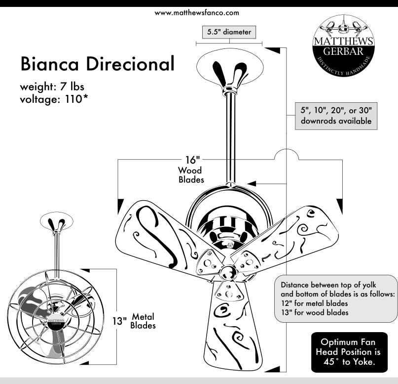
The Bianca Directional can be mounted with any one of the following downrod lengths: 5, 10, 20 or 30".
