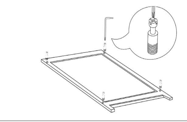
3) Align Right and Left Side Panels to the Back Panel and connect them together. Use a Slotted screwdriver or Phillips screwdriver to tighten the Cam Inserts. Slide the Bottom Board as shown below.
