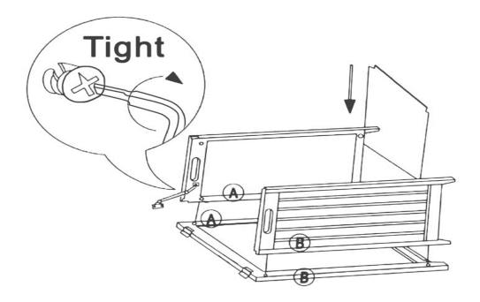
4) Align Front Panel (Flat Style shown below or Bowed Front Style) to the Side Panels and connect them together using a Slotted screwdriver or Phillips screwdriver.
