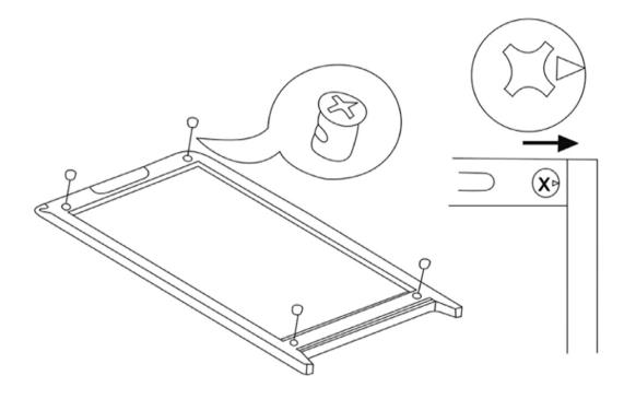
2) Insert 4 Threaded Posts into the four corner of the Front Panel. Also insert 4 Threaded Posts into the four corners of the Back Panel.
