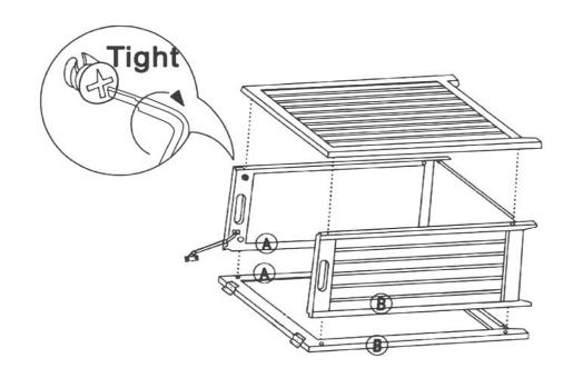
5) Align Hamper Lid to the Back Panel using the four Screws for Hinges provided with a screwdriver to tighten. Connect the Piano Hinge to the Hamper Lid (see diagram) using the two Screws for Piano Hinge with a screwdriver. Insert Interior Bag into the hamper (see diagram). Close the lid and you are done. Congratulations on your new hamper!
