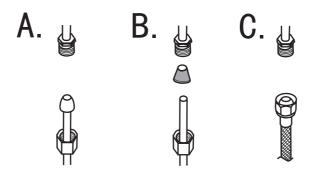
Connect to water supply lines with either:
