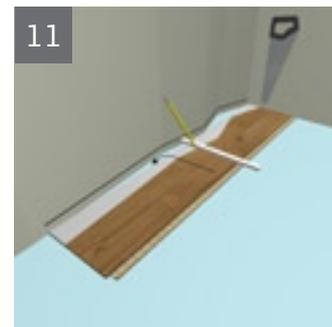
**12.** Drill holes in the board to accommodate heating pipes. The holes must be at least 20 mm larger than the pipe's diameter. Make saw cuts as shown in the diagram. When the board is fitted, the sawn piece needs to be glued in place and the holes covered with pipe collars.
