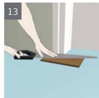
**13.** If you have to cut a door architrave, use a floorboard as a base so you get exactly the right height. If you need to knock a board along its length, protect the board's joint with a cut piece from a short end inserted into the joint.
