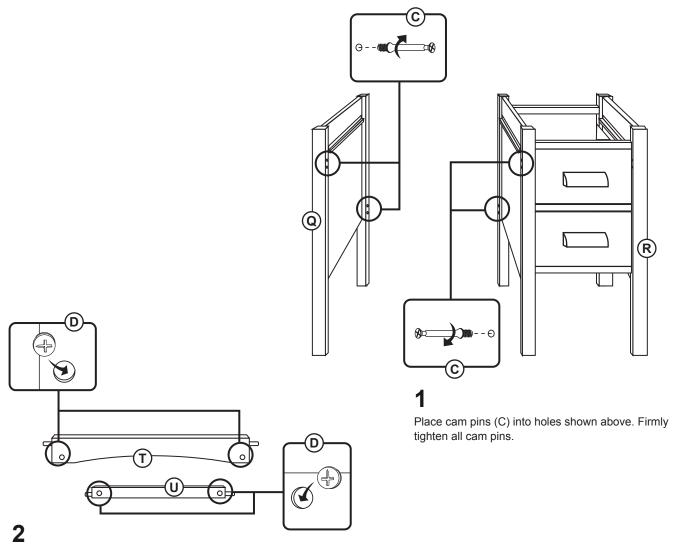
Place cam nuts (D) into holes on Parts T and U so that the arrow on the cam face is lined up with the opening.
