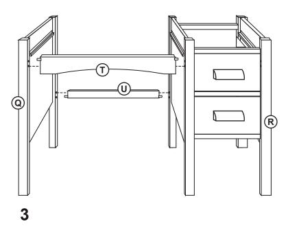
Once Parts T and U are attached to Parts Q and P, tighten cam nuts by turning clock-wise until they've locked into place.
