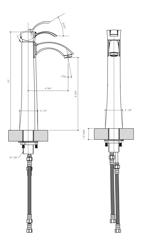
VG03023 THE MEASUREMENTS IN INCHES ARE ROUNDED TO THE NEAREST  $1/8^{\circ}$
